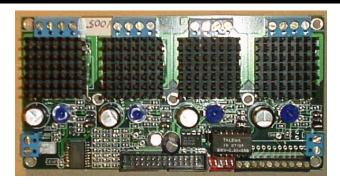
The XS-3525/8S-4 microstepping stepper motor driver is the perfect choice for CNC retrofitting of desktop and small benchtop milling machines. Connect bipolar wired stepper motors, power, and a parallel port signal source
